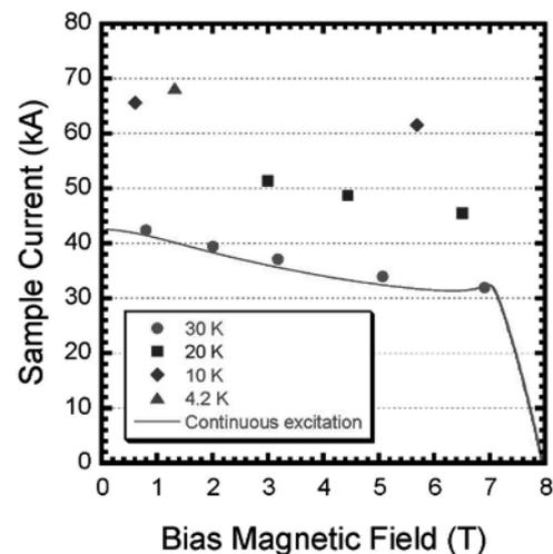
Fig.1 Critical currents of the HTS conductor sample measured at various temperatures as a function of the bias magnetic field (perpendicular to the *c*-axis of the GdBCO tape). The current observed in the continuous excitation in Fig. 2 is also plotted.
