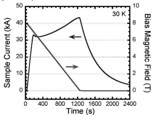
Fig.2 Temporal evolutions of the current of the HTS conductor sample and the bias magnetic field observed in the continuous excitation.
