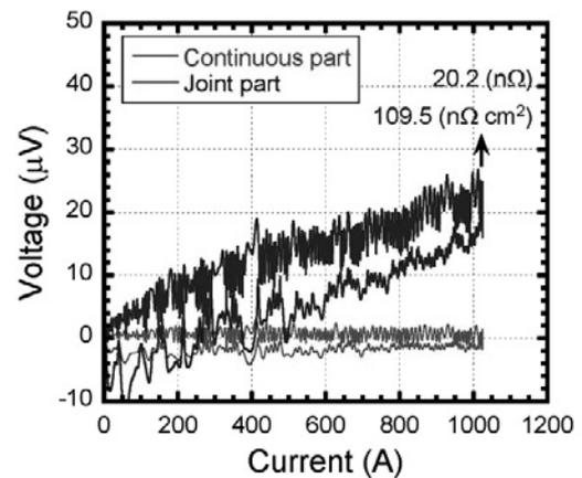
Fig. 1 Joint voltage of the 10-kA class soldered lap joint as a function of current.
