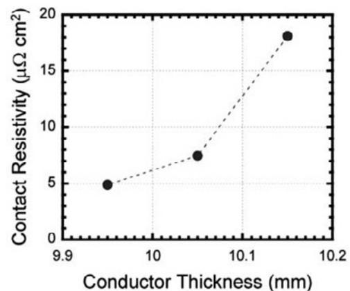
Fig. 2 Contact resistivity obtained by the 10-kA class sample in mechanical lap joint as a function of the conductor thickness.
