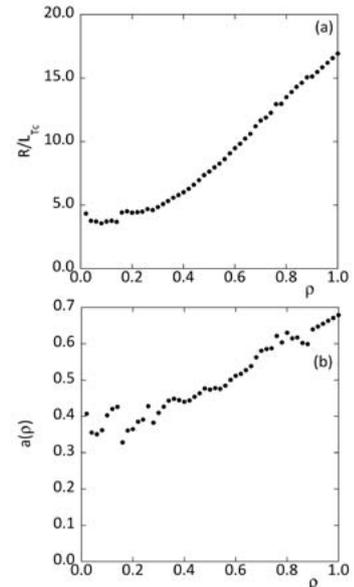
Fig. 1: The radial dependence of (a) the critical ion temperature gradient  $R/L_{T_c}$  and (b) the slope  $a(\rho)$  in modeled ion diffusivity
