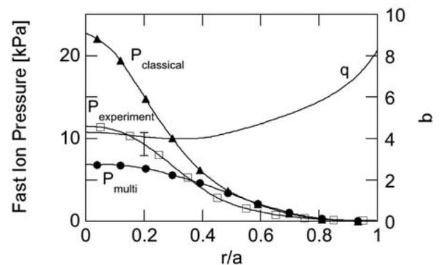
Fig. 2 Comparison of fast ion pressure profile among multi-phase simulation (circle), classical (triangle) simulation, and experiment (square) with an error bar shown in the figure.
