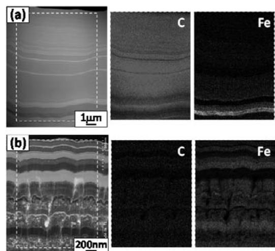
Fig. 1. Cross-sectional BF-TEM images and corresponding EDS mapping images of C and Fe inside the dashed square lines in BF-TEM images. (a): from divertor tile, (b) from first-wall
