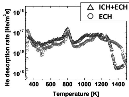
Fig. 2. TDS spectrum of helium from the SUS316L specimens after exposed to the ICH+ECH discharge cleanings and the ECH discharge cleanings.
