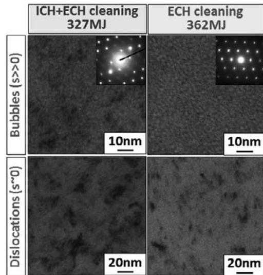
Fig. 1. TEM images of the SUS316L specimens and corresponding electron diffraction pattern after exposed to the ICH+ECH discharge cleanings with the total input power of around 327 MJ to the plasma and the ECH discharge cleanings with the total input power of around 362 MJ to the plasma.
