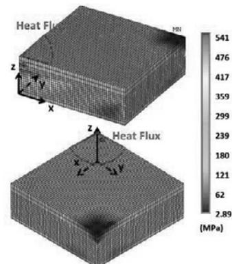
Fig. 2. Von Mises stress in the dimension of 5 mm x 5mm x 1.6 mm near the interface in the sample corresponding to experimental condition (1)
