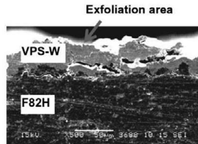
Fig. 1. SEM image of cross section after heat loading of experimental condition (3)
