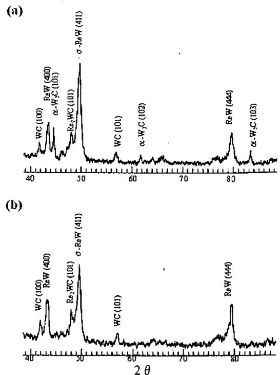
Fig. 1 X-ray diffraction analysis near joint interface annealed for 1.8 ks at 1800°C(a) and 1.8 ks at 2000°C(b).
