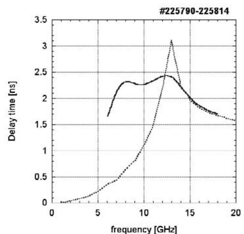
Fig. 3. Observed delay time as a function of launching frequency (solid line) and estimated one (dotted line).
