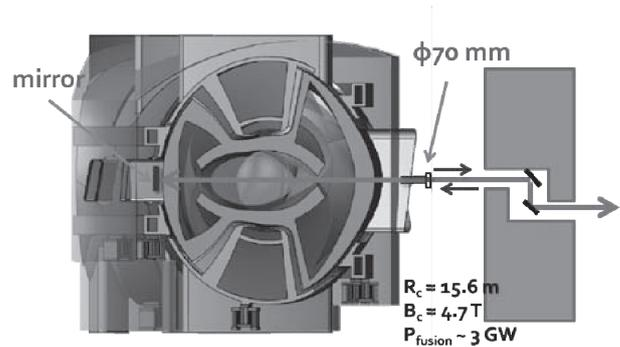
Fig. 1. Example of accessibility for microwave diagnostics in future fusion reactor (FFHR-d1).
