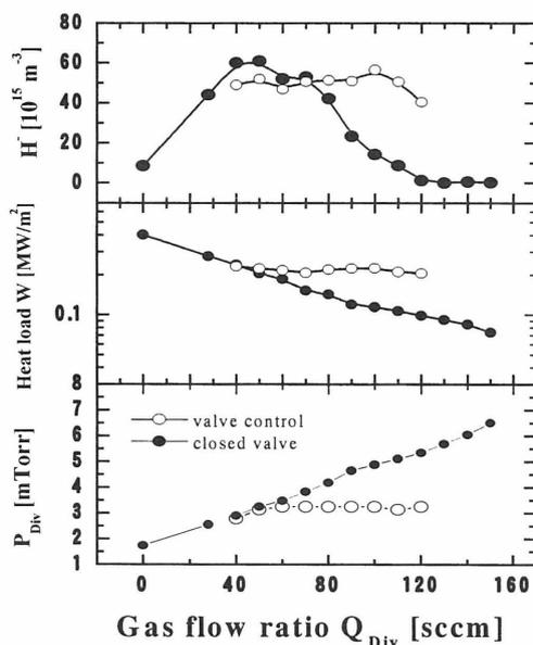
Fig.2 Typical characteristics of  $P_{Div}$ ,  $W$  and  $H^-$  on the gas flow ratio  $Q_{Div}$ .
