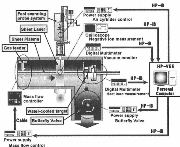
Fig.1 Schematic diagram of control system.
