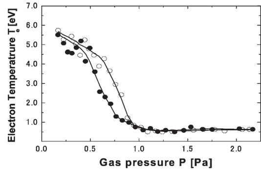
Fig. 2 Dependence of hydrogen gas pressure P on the electron temperature  $T_e$  at a discharge current of 50A. The geometry of the target plates are the oblique target ( $\circ$ ) and the V-shaped target ( $\bullet$ ).
