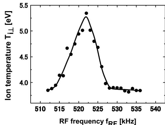
Fig.1. Ion temperature  $T_{i\perp}$ , plotted for various RF frequencies at a power supply of 300 W.
