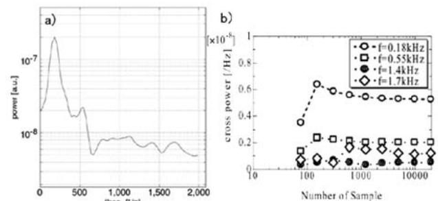
Fig. 3. a) The averaged power spectrum of low frequency range (0-2000Hz). b) The convergent of auto power in each power peak.
