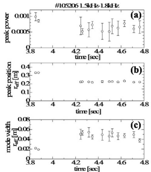
Fig. 2: The summary of the transition of the mode structure. (a) the peak power of the 1.5 - 1.8kHz electron temperature fluctuation. (b) the peak position. (c) the mode width calculated from the  $\xi$  profile.
