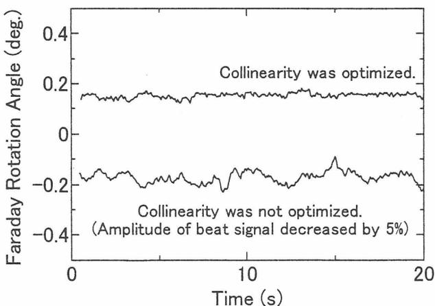
Fig. 1 Comparison of baseline fluctuations of the Faraday rotation angle.
