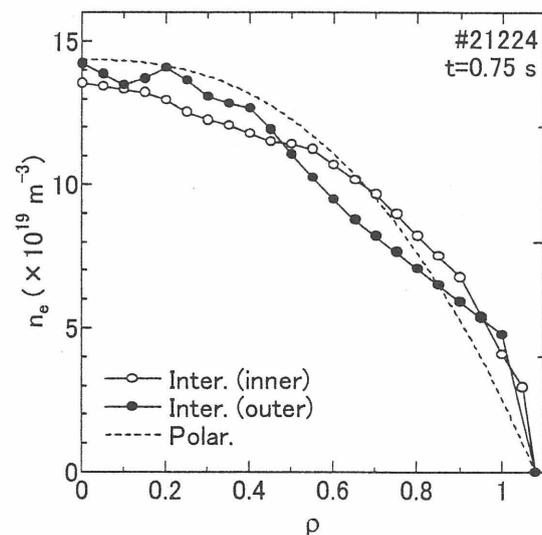
Fig. 3 Comparison of the electron density profile estimated from the 3-ch polarimeter with those from the 13-ch interferometer.
