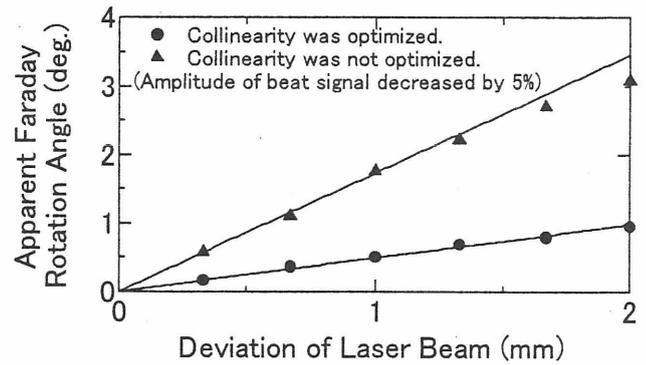
Fig. 2 The apparent Faraday rotation angle shifts with laser beam deviation.
