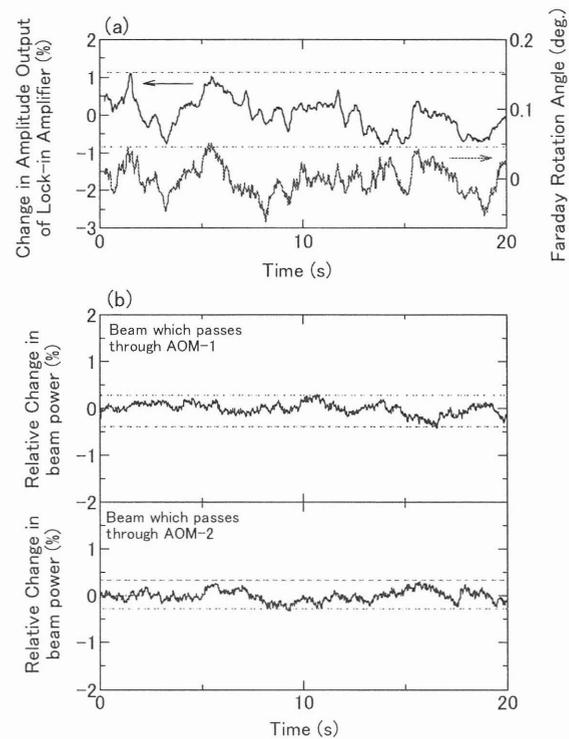
Fig. 1. Time traces of the relative amplitude of the beat signal and the Faraday rotation angle simultaneously measured with a lock-in amplifier (a) and those of relative beam powers of counter-rotating polarized beams (b).
