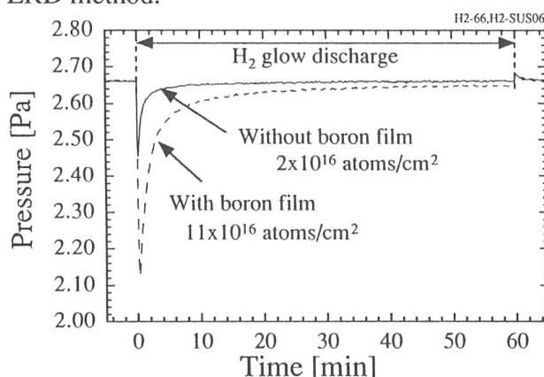
Fig.1. Time evolution of total pressure (=H<sub>2</sub> pressure) during H<sub>2</sub> discharge with and without B films.
