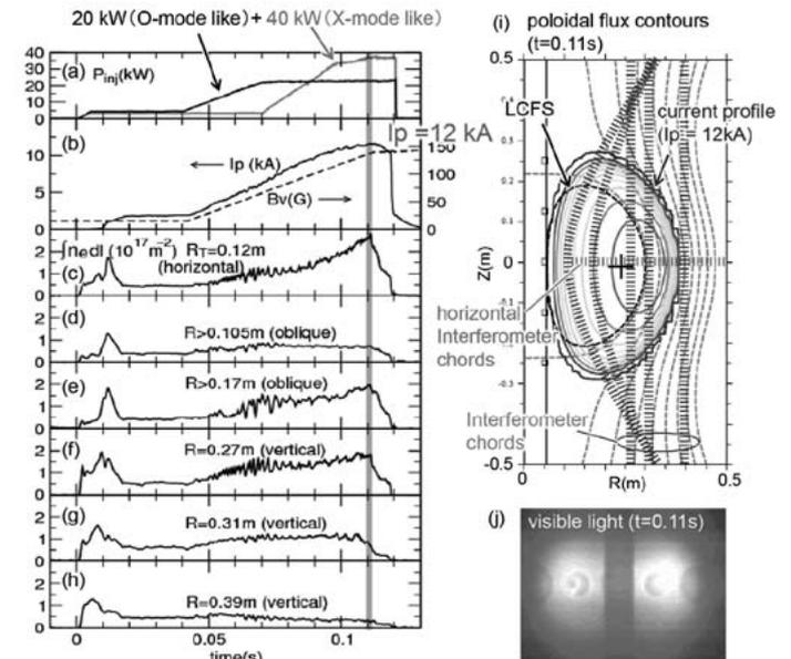
Fig. 1.  $I_p$  reaches 12kA and the line-average density exceeds seven times the cutoff density
