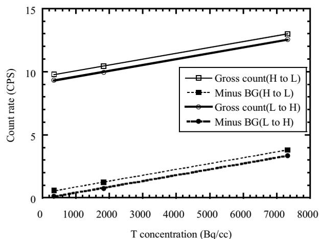
Fig. 2. Measurement of tritium in water by the plastic scintillator. H and L mean high and low concentration respectively.
