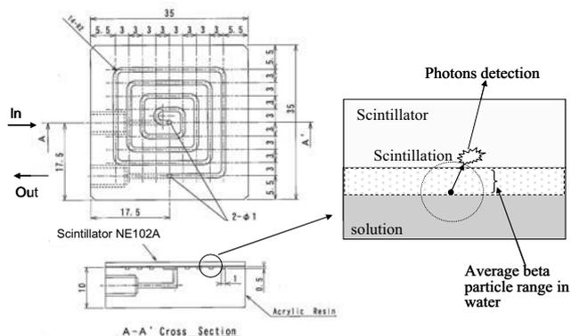
Fig. 1. An equipment of tritiated water flow presumed to be collected from air sampling system and detection image by plastic scintillator.
