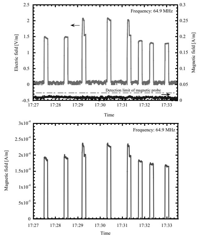
Figure 2 Electric and magnetic field leakage around the ICRF source devices. Upper(1) is measured by EMC300 and lower (2) was measured by SRM-3000
