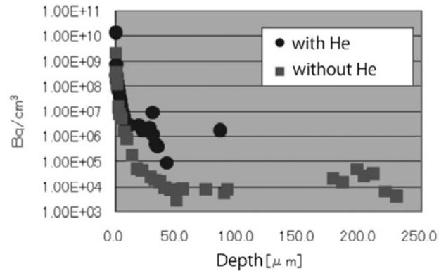
Fig. 1 Depth profiles of Tritium for the samples with and without He plasma exposure.
