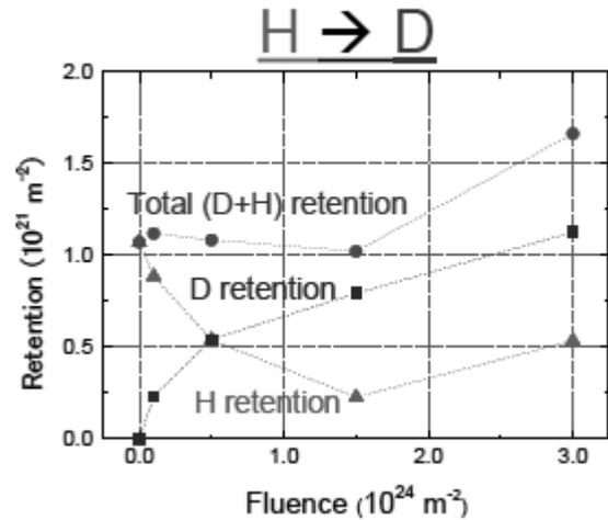
Fig. 2 Evolution of retention as a function of post fluence. Pre-irradiation species is H and post-irradiation species is D at 473 K.
