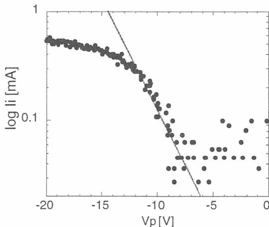
Fig. 1 Voltage-current characteristic curve of ISP obtained in NAGDIS-II helium plasma. The magnetic field is 0.2 T, the electron density and temperature are  $5 \times 10^{18} \text{m}^{-3}$ .
