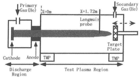
Fig.1. Schematic of experimental apparatus NAGDIS-II.
