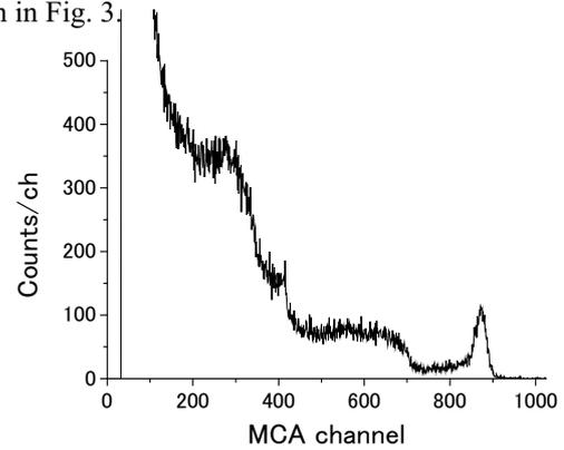
Fig. 1. An example of response function for 14 MeV neutrons obtained by a CVD single crystal diamond detector made by Hokkaido University.
