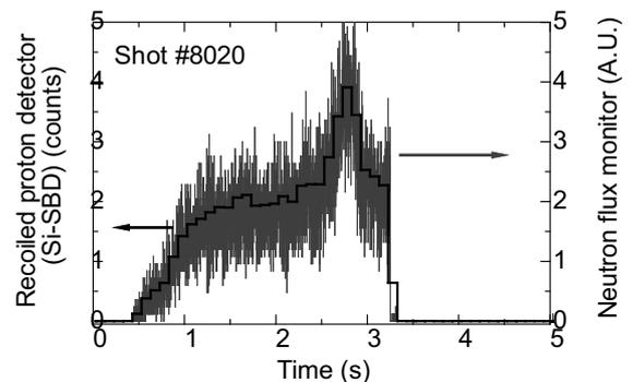
Fig.3. Time traces of count rate of Recoil Proton Detector and signals of KSTAR neutron flux monitor.
