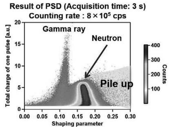
Fig. 3 An example of the neutron-gamma ray discrimination.
