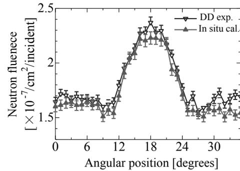
Fig. 1 Neutron fluence distribution near the O-port of LHD.
