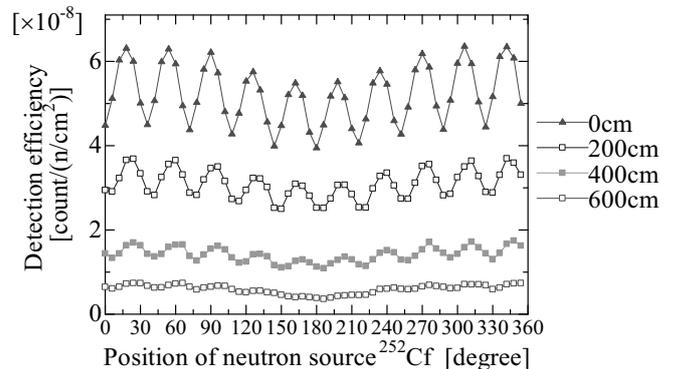
Fig. 2 Detection efficiencies of a fission chamber placed on the center axis and at 0, 200, 400, 600 cm from the equatorial plane of the LHD.
