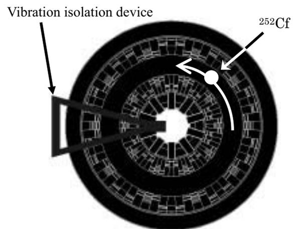
Fig. 1 Simplified geometry of the LHD for neutron transport simulations.
