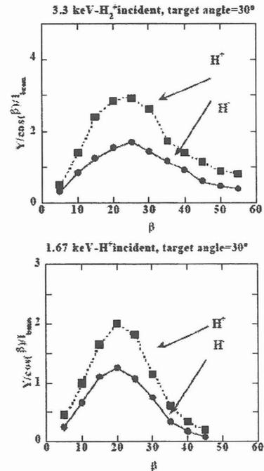
Fig. 1. Graphs showing (a), the angular distribution of the negative ion yield and the positive ion yield due to incident molecular hydrogen ions, and (b), those due to incident proton at the same velocity.
