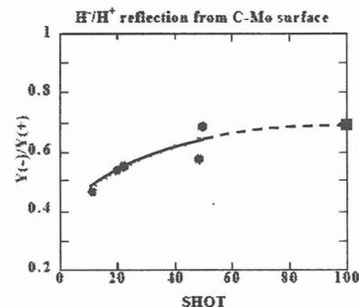
Fig. 2. Evolution of the ratio of negative ions to positive ions reflected from carbon coated Mo surface. As the number of shots proportional to the ion dose increases, the ratio approaches the value of the pure Mo.
