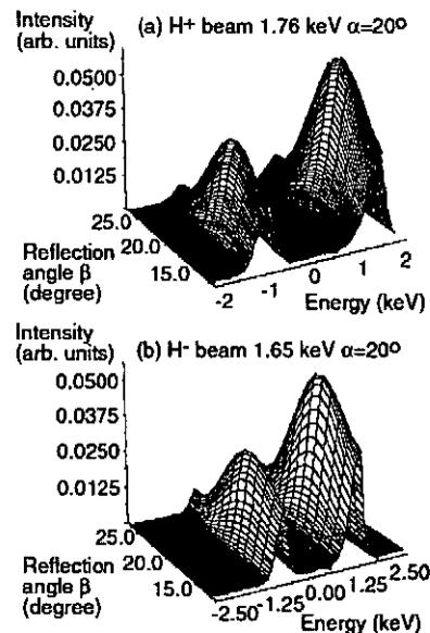
Fig. 2. Examples of energy and angular resolved intensity profiles of  $H^+$  and  $H^-$  ions reflected from Mo surface at the incident angle of  $20^\circ$  for (a)  $H^+$  and (b)  $H^-$  beam injection.
