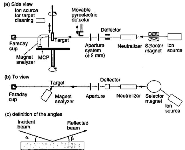
Fig. 1. Schematic diagram of the experimental setup with definitions of incident and reflection angles.
