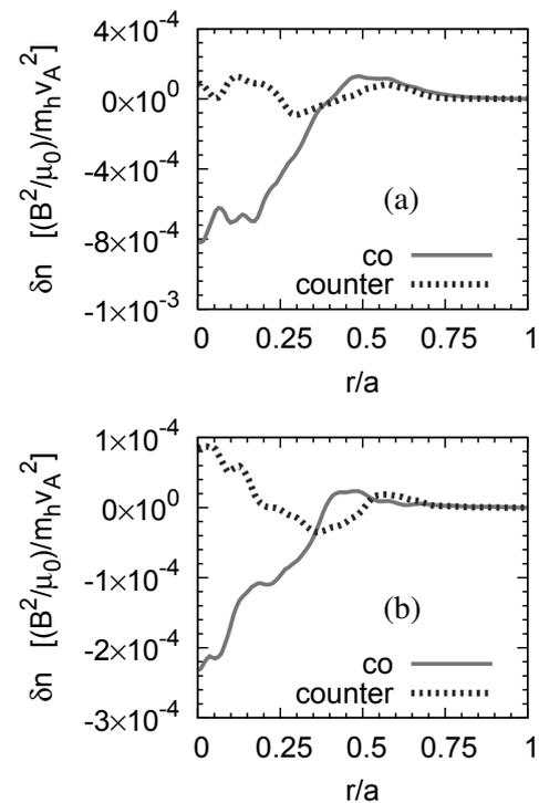
Fig. 1: Comparison of energetic particle density profile perturbations between (a) RSAE mode for  $q_{min} = 1.95$  and (b) TAE mode for  $q_{min} = 1.875$ . Co-going particles to the plasma current are transported by the RSAE mode; whereas both the co- and counter-going particles are transported by the TAE mode.
