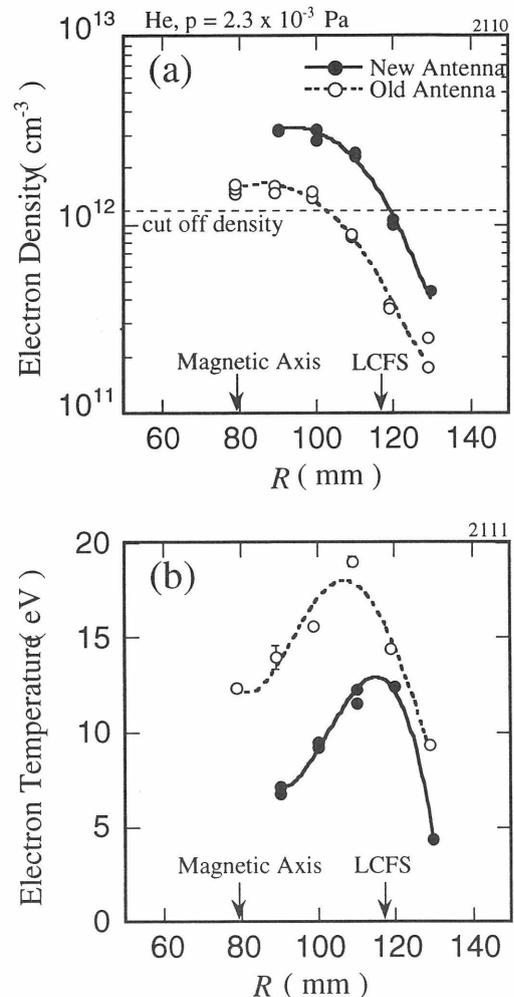
Fig.1 Radial profiles of (a) the electron density and (b) the electron temperature measured with the triple probe.
