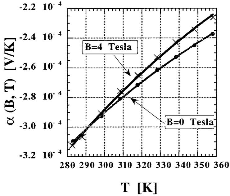
FIG. 5. Thermoelectric power of InSb sample as a function of temperature. The crosses represent experimental results at  $B = 0$  Tesla. The filled circles indicate the experimental results at  $B = 4$  Tesla. The solid curves are guide for eyes.
