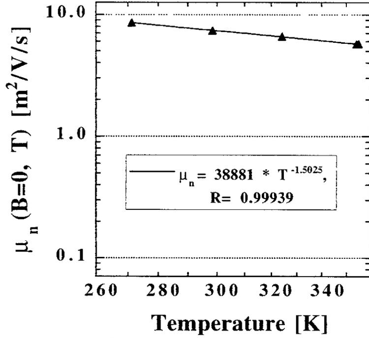
FIG. 8. Temperature dependence of the electron mobility. The experimental results are fitted by  $\mu_n \approx 7.5 \times (T/300)^{-1.50} [\text{m}^2/\text{V}/\text{s}]$ .
