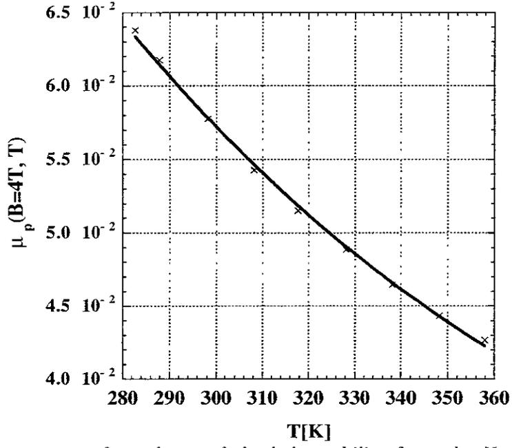
FIG. 9. Temperature dependence of the hole mobility from the Nernst coefficients. The experimental results are fitted by  $\mu_p(B = 4\text{Tesla}) \approx 0.065 \times (T/300)^{-1.7}$  [ $\text{m}^2/\text{V}/\text{s}$ ].
