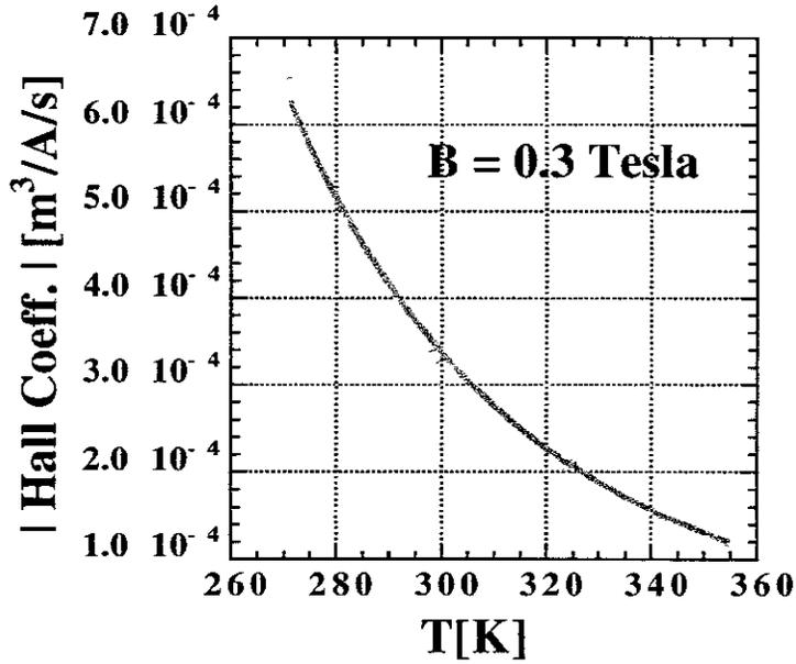
FIG. 3. Resistivity (a) and Hall coefficient (b) of InSb sample as a function of temperature. The closed circles indicate the experimental results. The solid curve is a guide of eyes.
