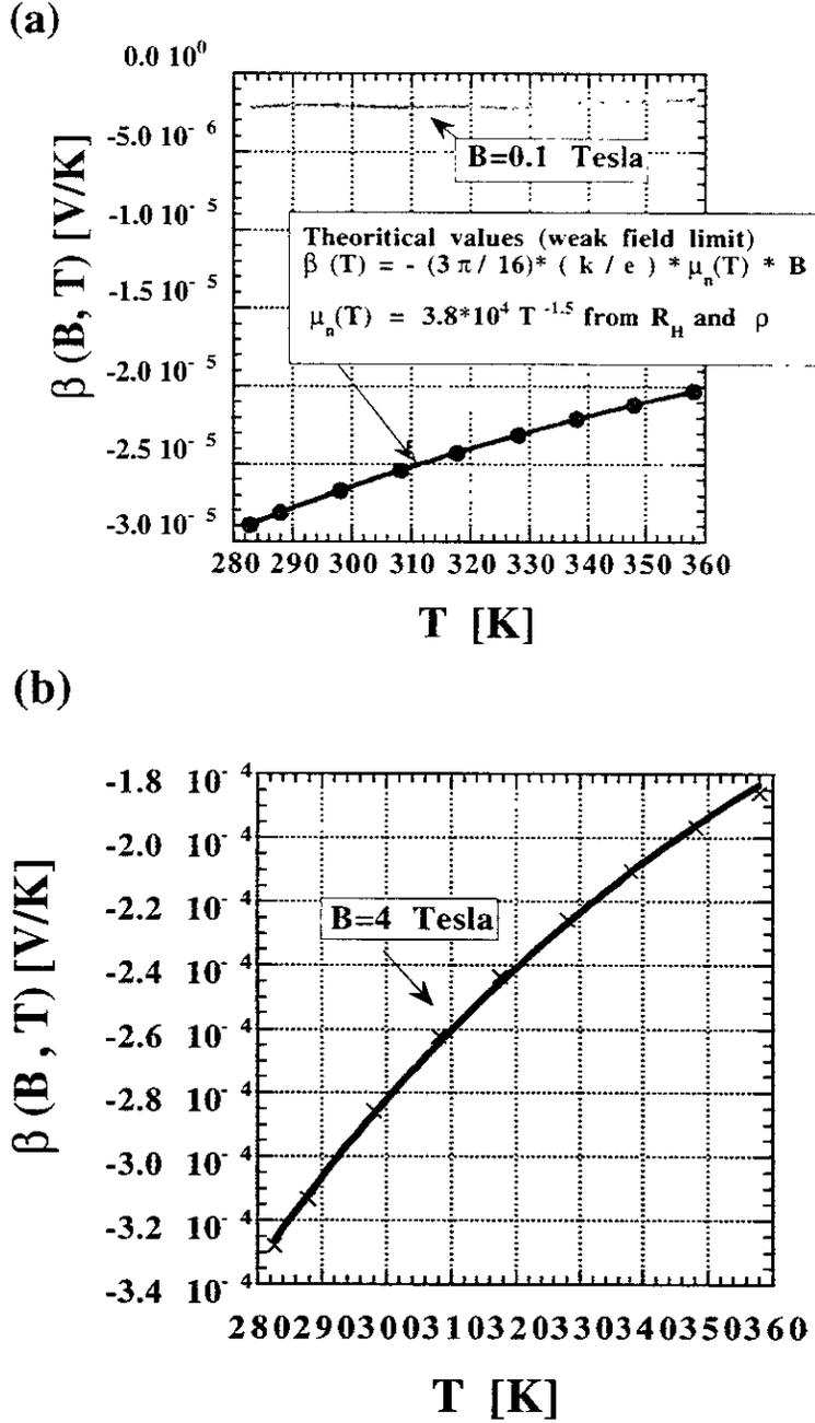
FIG. 6. Plot of Nernst effects,  $\beta = N \times B$  in the case of  $B = 0.1$  Tesla (a) and 4 Tesla (b). The crosses indicate the experimental results. The filled circles in Fig. 6(a) were calculated by the single band model with the mobilities which were given from the Hall coefficients and resistivities. In Fig. 6(b), the solid curve is given by the least square method.
