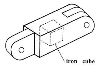
Fig. 2(c) One piece of the chain. Magnetic monopoles are trapped on the surfaces of the iron cube which is buried inside a nonmagnetic stainless steel (SUS 304) block with joints at both sides.
