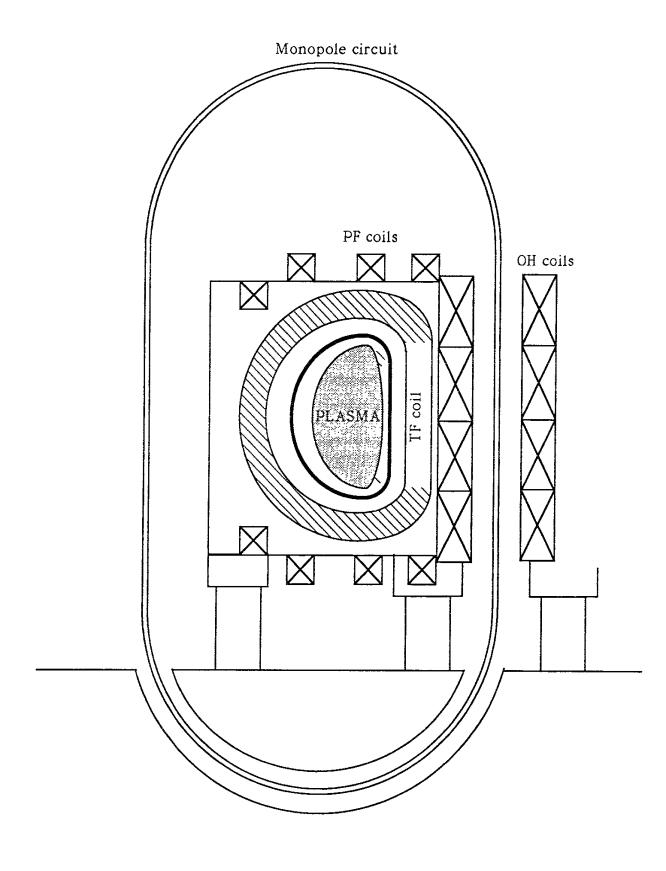
Fig.2. (a) A next generation tokamak equipped with a magnetic monopole circuit.
