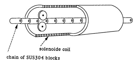
Fig. 2(b) A section of the magnetic monopole circuit. A chain of the stainless steel blocks is housed in a solenoide coils in which the magnetic field intensity is controlled so that the magnetic force on the chain balance with the frictinal force.
