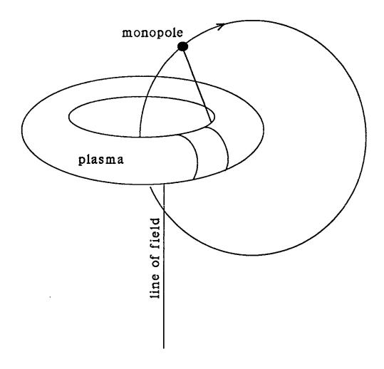
Fig.1. A field line behavior as a magnetic charge circulates along a circuit which intrelinks a toroidal plasma. The magnetic charge winds field lines along the toroidal plasma infinitely thereby generating a loop voltage equal to the circulation frequency times the magnetic charge.
