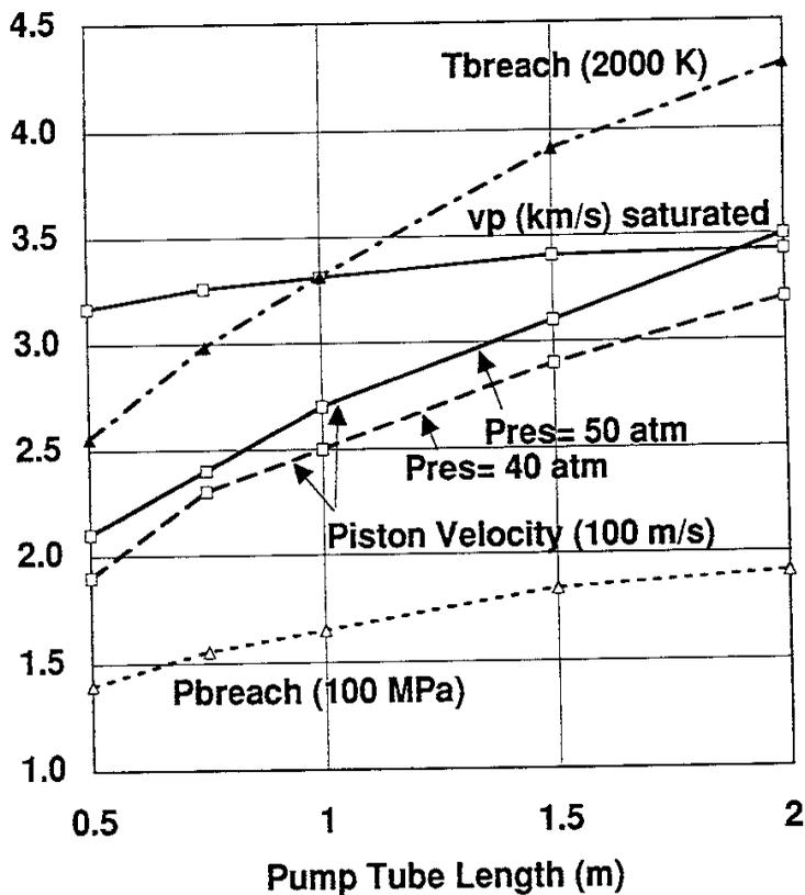
Fig. 4(b) Dependence of the breech pressure, temperature, piston velocity, achievable pellet velocity on the code .
