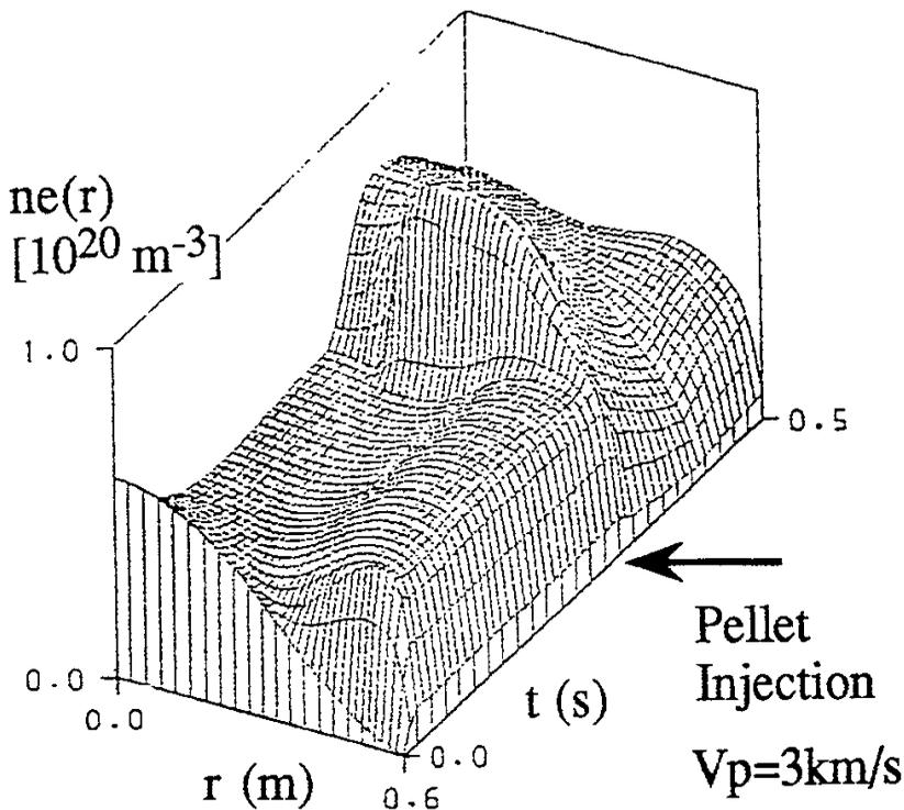
Fig.1 One example of simulation results of pellet ablation.
