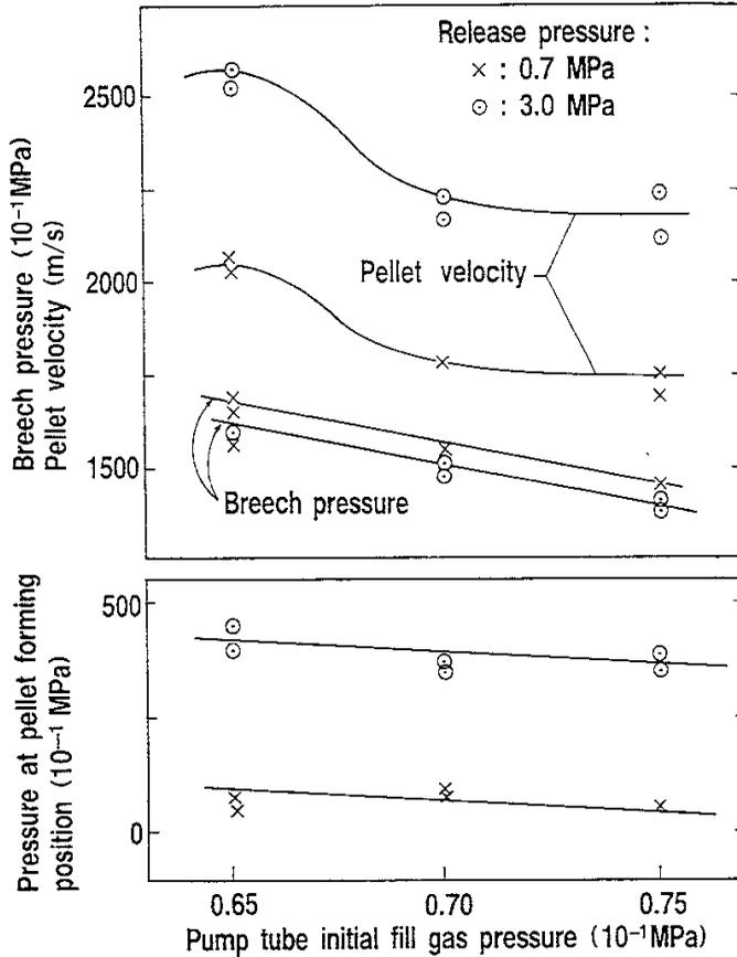
Fig. 6 Dependence of breech pressure and pellet velocity on pellet release pressure. For this experiment only, a nylon pellet of 12 mg is used. Piston mass, pump tube length, and reservoir pressure are 20.4 g, 0.75 m, and 4 MPa, respectively.
