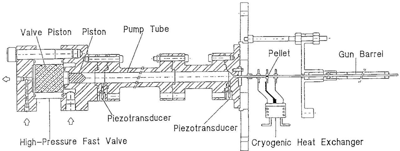
Fig. 2 Schematic of two-stage gas gun with the originally made high conductance fast valve.
