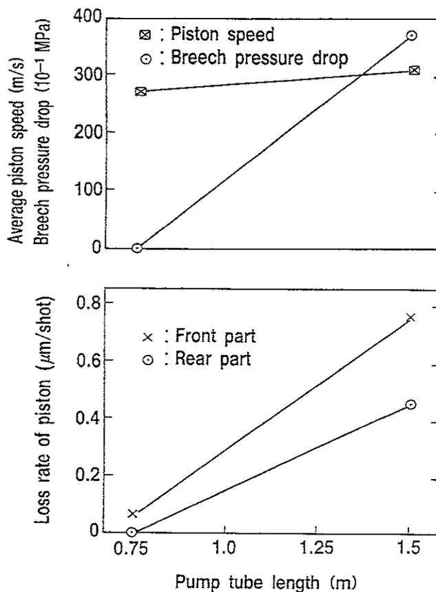
Fig. 4(a) Loss rate of the piston diameter for 0.75 m and 1.5 m pump tubes. The hardness for the former and the latter are 432 Hv and 388 Hv, respectively.
