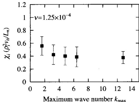
FIG. 4: Ion heat transport coefficient  $\chi_i$  for different truncation wave numbers  $k_{\max}$  with  $\nu = 1.25 \times 10^{-4}$ .
