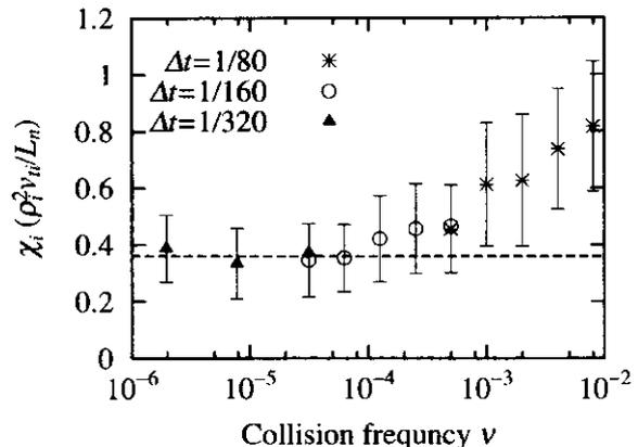
FIG. 3: Anomalous ion heat transport coefficient ( $\chi_i$ ) for different collision frequency  $\nu$  averaged from  $t = 1000$  to 3000. A horizontal dashed line represents  $\chi_i$  for  $\nu = 0$ .
