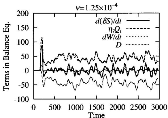
FIG. 2: Time-history of each term in Eq.(4),  $d(\delta S)/dt$ ,  $dW/dt$ ,  $\eta_i Q_i$ , and  $D$  for  $\nu = 1.25 \times 10^{-4}$ , where data are running-averaged for a time period of  $\tau = 50$ .
