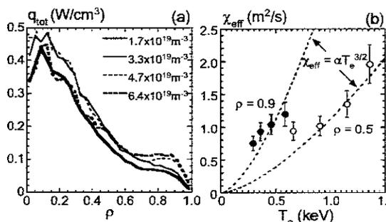
Fig.5 (a) Profile of power deposition from NBI in the discharges in the case with  $R_{ax}=3.75$ m. (b) Temperature dependence of thermal diffusivity at two radii of  $\rho=0.5$  (open circles) and  $\rho=0.9$  (solid circles) derived from the power balance.
