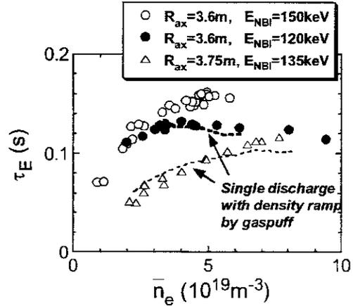
Fig.1 Dependence of energy confinement time on density. Closed circles:  $R_{ax}=3.6$  m,  $P_{NBI}=4.7$  MW,  $E_{NBI}=120$  keV. Open circles:  $R_{ax}=3.6$  m,  $P_{NBI}=4.3$  MW,  $E_{NBI}=150$  keV. Open triangles:  $R_{ax}=3.75$  m,  $P_{NBI}=4.1$  MW,  $E_{NBI}=135$  keV. Dotted lines: traces of the single discharges with density ramp-up.
