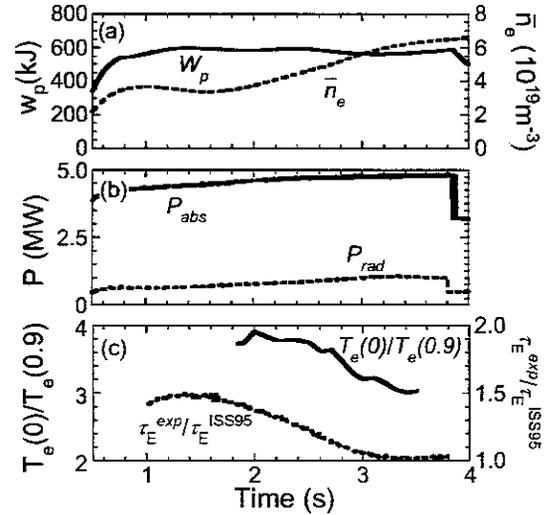
Fig.2 Waveforms of the discharge with density ramp-up in the case with  $R_{ax}=3.6$  m,  $P_{NBI}=4.7$  MW,  $E_{NBI}=120$  keV. (a) Stored energy and line averaged density. (b) Absorbed power of NBI and total radiation power. (c) Ratio of the central electron temperature to that at  $\rho=0.9$  and improvement factor of energy confinement time on ISS95.
