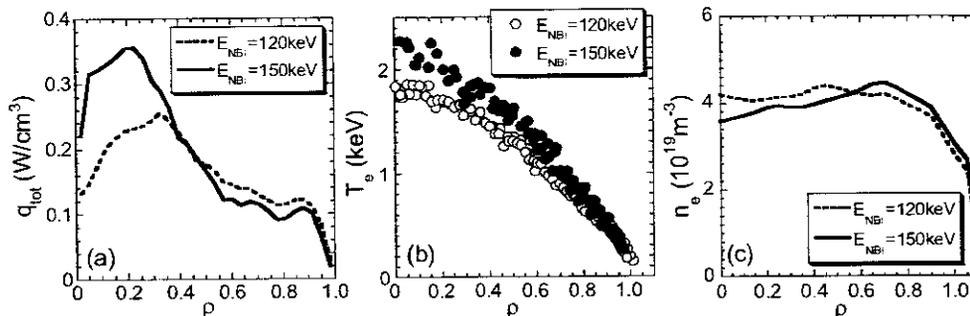
Fig.6 Plasma profiles in discharges with different NBI conditions. (a) Heat deposition. (b) Electron temperature. (c) Electron density. Dotted lines and open circles:  $P_{NBI}=4.7$  MW,  $E_{NBI}=120$  keV (#28168). Solid lines and closed circles:  $P_{NBI}=4.3$  MW,  $E_{NBI}=150$  keV (#28936).
