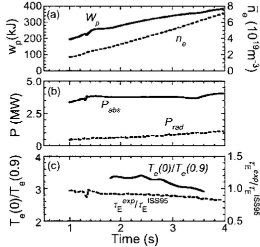
Fig.3 Waveforms of the discharge with density ramp-up in the case with  $R_{ax}=3.75\text{m}$ .  $P_{NBI}=4.1\text{MW}$ ,  $E_{NBI}=135\text{keV}$ . (a) Stored energy and line averaged density. (b) Absorbed power of NBI and total radiation power. (c) Ratio of the central electron temperatures to that at  $\rho=0.9$  and improvement factor of energy confinement time on ISS95
