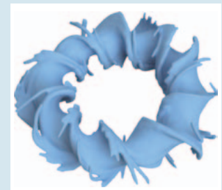
Fig. 2 The 3D model of the plasma shape generated from specialized Marching cubes method.
