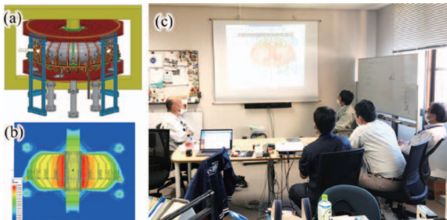
Fig. 2 Technical cooperation program: (a) 3D-CAD model of RELAX; (b) distribution of magnetic field in a vertical section; (c) technical discussion regarding the modification of magnetic field coils.
