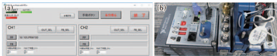
Fig. 2 Voltage waveform output system: (a) GUI and (b) hardware (CompactRIO, product of National Instruments).
