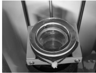
Fig. 2 Photos of the active tritium sampling system without combustion gases and setup of the cylindrical water vial
