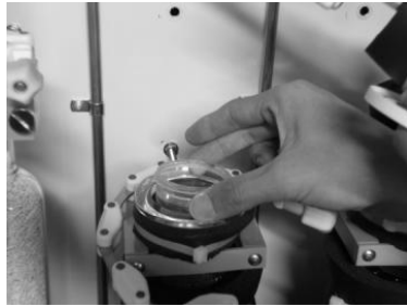
Fig. 2 Photos of the active tritium sampling system without combustion gases and setup of the cylindrical water vial
