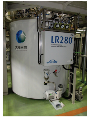
Fig. 2. Photograph of the variable temperature helium refrigerator/liquefier.
