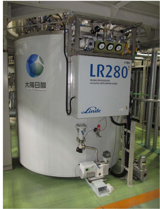
Fig. 2. Photograph of the variable-temperature helium refrigerator/liquefier.
