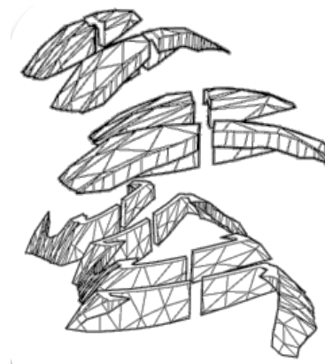
Fig. 6. (a) Top view of the T-SHELL blanket (i.e., toroidally sliced tritium-breeding blanket). (b) Bird's-eye view of the horizontally sliced neutron shield blanket.
