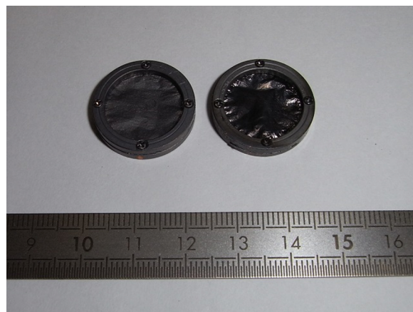
FIG. 3. Platinum foil samples blackened by carbon spray (left) and vacuum evaporation (right).
