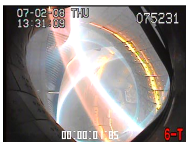
Figure 2: Example of the light reflected from the divertor tiles
