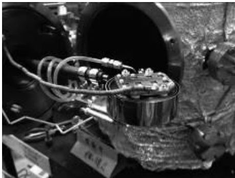
Fig. 1. Photograph of manufactured sample holder. The gas can be introduced through pores near samples.
