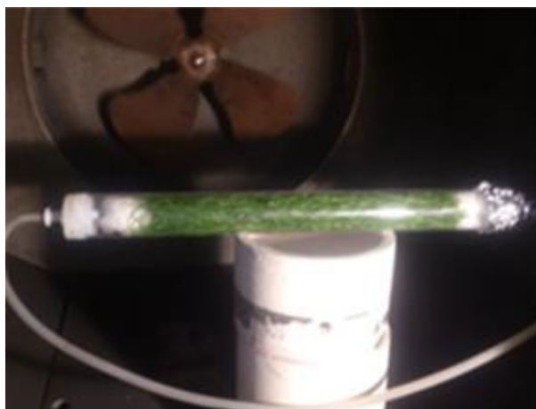
Fig. 2 Setup of quartz tube with pine needle samples in test furnace.
