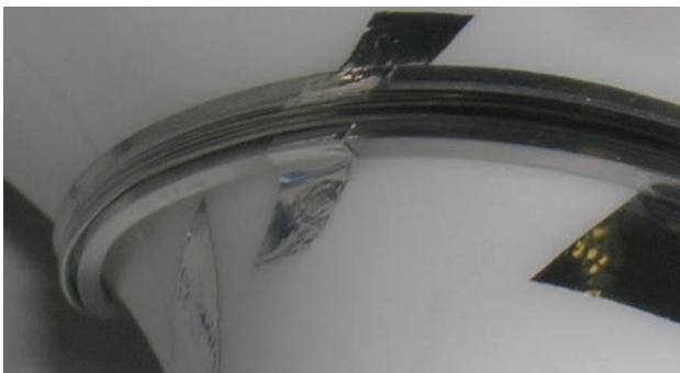
Fig. 7 Trial of helical winding. The wire is wound in the grooves by three turns.
