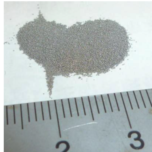
Fig. 2 The getter material of Fe-5at%Ti alloy pebbles.
