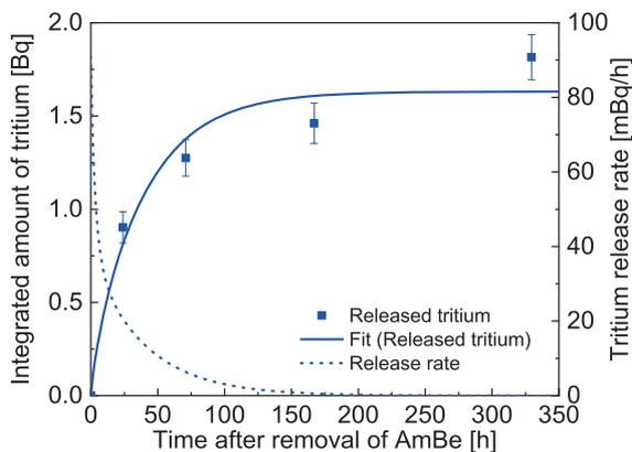
Fig. 5 Integrated amounts of tritium recovered after the AmBe neutron source was removed [11].
