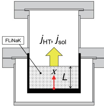
Fig. 3 Calculation model of tritium release from FLiNaK in a one-dimensional diffusion equation.
