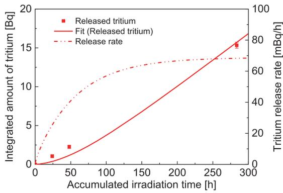
Fig. 4 Integrated amounts of tritium recovered after the AmBe neutron source was placed [11].
