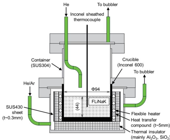
Fig. 2 Cross-section of FLiNaK container (unit: mm).
