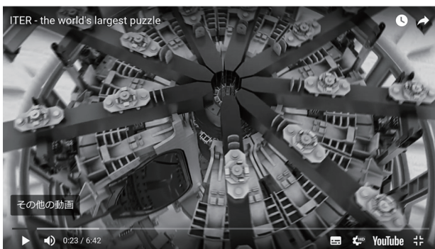
Fig. 2 Assembly of TF coils and VVs of ITER. Space for the last component is open [1].
