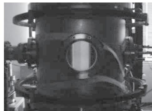
Fig. 3. 2.45GHz-ECH He plasma production in TOKASTAR-2. Plasma light with inner vertical limiter stripe is shown between two TF coils
