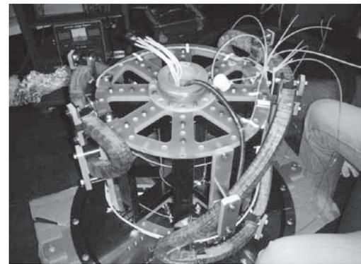
Fig. 2. Toroidal, poloidal and helical coil systems of TOKASTAR-2 installed inside the cylindrical vacuum chamber
